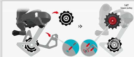
Remove the lower pulley from the original derailleur. When installing the AOPW lower pulley, align the STOP PIN on the pulley cap with the specified position on the cage, as shown in the illustration. Once the lower pulley and cage are properly aligned, reattach the fixing screw.
