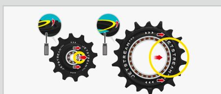
Apply one drop of TRIPEAK SUPRA LV Fluid to the bearing, then rotate it to evenly distribute the lubricant.
