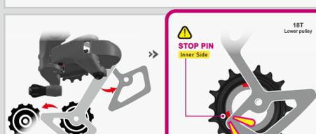
Tighten the upper and lower AOPW pulley fixing screws to the torque value recommended by the derailleur manufacturer.
