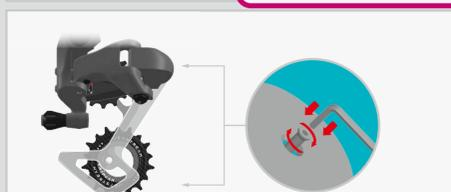
Reinstall the chain on the bike, ensuring that the narrow-wide teeth of the pulleys engage precisely with the chain's gaps during installation.
