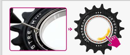
Carefully press the seal back onto the bearing, ensuring it is installed properly and securely.
